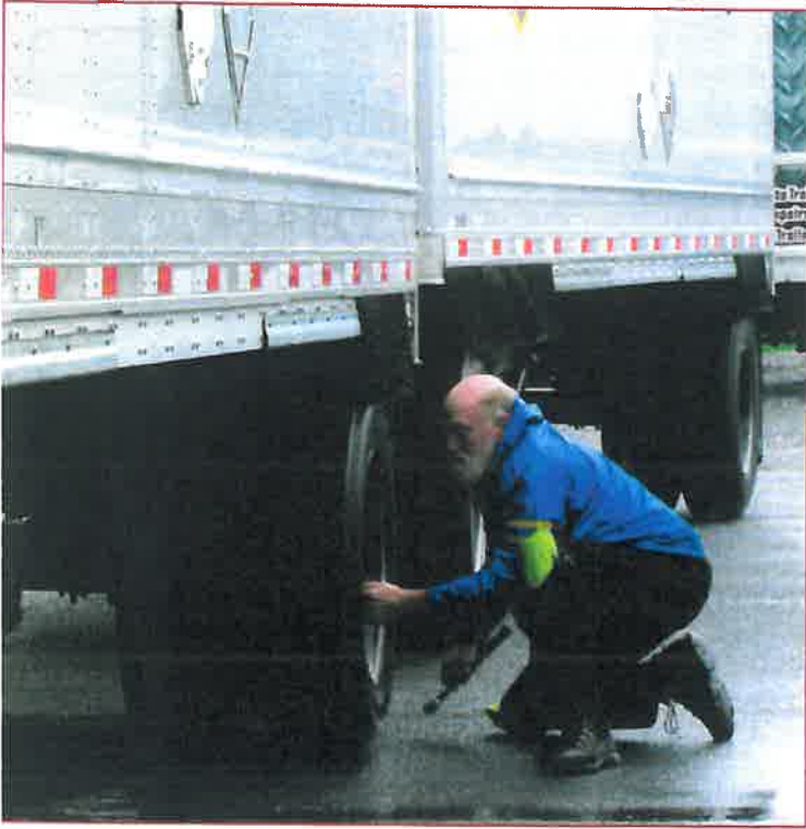
Puddles or no puddles, to do a proper pre-trip inspection, you have to look under the truck, in the wheel wells, and around the tires.
